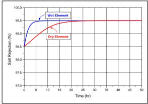
1. CSM RO elements could be supplied either wet or dry.
