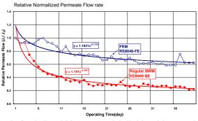
The flux decline of CSM FRM is only half of that of the general brackish water RO membrane under the condition of zero liquid discharge system.
