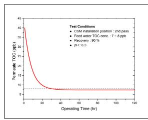
TOC reduction in CSM UPW products used in the  $2^{\rm nd}$  pass ultrapure water system. Rinse down time may vary according to the feed water conditions.
